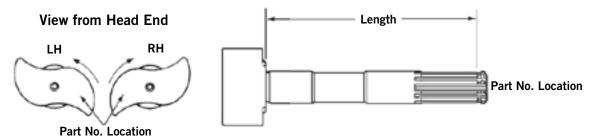
LH and RH indicates only the direction of cam rotation; NOT which side of the vehicle the cam is used on. LH = (Counterclockwise) RH = (Clockwise) NOTE: Not all camshaft lengths are measured to the beginning of the snap ring groove.
